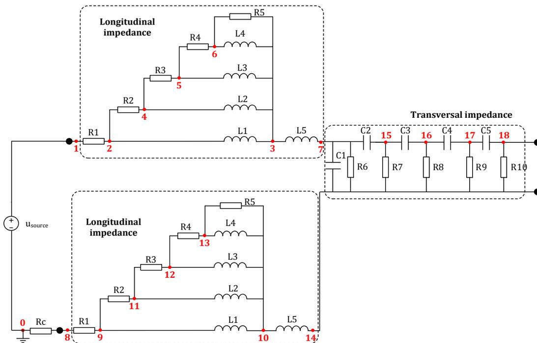
**Fig. 2.1. Single cell equivalent circuit considering the longitudinal and transversal impedances.**
