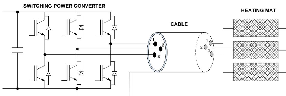
**Fig. 1.1. Power electronic converter, power cable and heating mat.**
